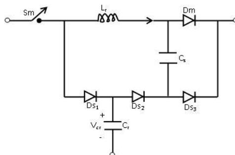
Fig (3.1) passively soft switching circuit cell
